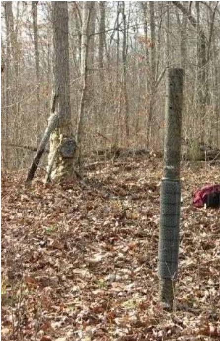
Remote camera and Gauthier hair pole set up at LBL. The pheromone lure is hung inside the PVC pipe.
